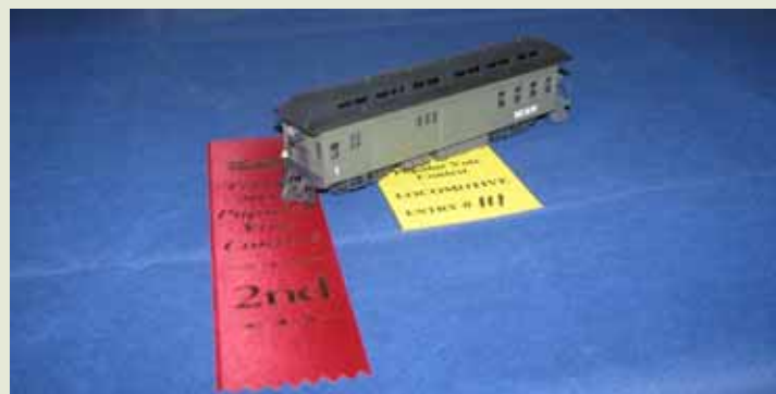
HO scale Kit bashed motor car MDC combine powered with a Brill trolley mechanism by Phil Holden
