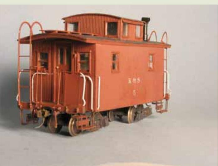
The painted caboose before final weathering and paint touch-up. The end ladders are held down by brass pins in the end beam and roof. A functioning door is simply hung on paper hinges, held with styrene cement.
