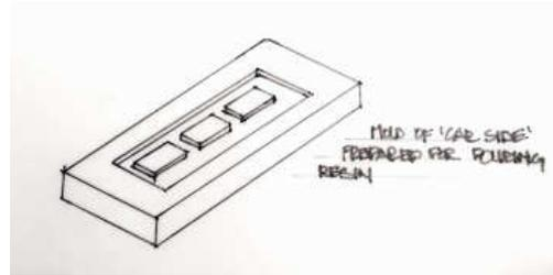
**Step 2:** Pour the plastic resin into the mold, overfilling slightly. This will help any bubbles floating on the surface get pushed out of the mold as the excess resin is squeezed out of the mold in the following step. Gently work the liquid resin into the details in the mold that might hold air bubbles with a toothpick, and pop any bubbles that gather on the surface or use the toothpick to push the bubbles to the edge of the mold.
