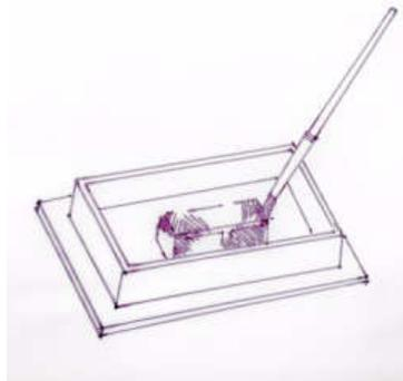
**Step 4** Allow the mold to cure for at least 16 hours, break the dam and peel the mold off the master.
