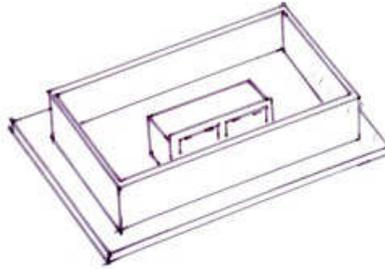
**Step 3** Pour in the silicone rubber mold material. Start by painting mold material onto the exposed detailed sides of the master part with an old paintbrush, watching for and removing any bubbles that get trapped in the surface details. When the part is covered with brushed on mold material and you're satisfied that you've removed any bubbles, pour in the remaining mold material. Any air bubbles in the mold material should float to the surface and not affect the quality of the mold.
