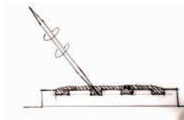
**Step 3:** Apply the top of the mold – Start at one end of the mold and 'roll' the top piece down from one end to the other, squeezing out the excess resin in the process. The mold protuberances that will form the openings (windows) in the casting will support the top of the mold. Molds with no windows are actually harder to cast consistently because pressure on the mold top piece tends to make the centre of the casting too thin.
